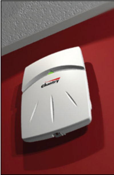
Wall mounted Beacon Point antenna
